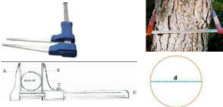
Gambar 1.26 Alat ukur diameter pohon
