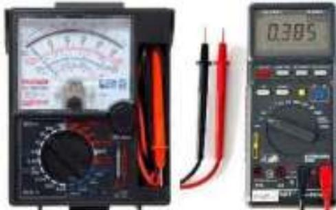
Gambar 4.18 Multimeter
