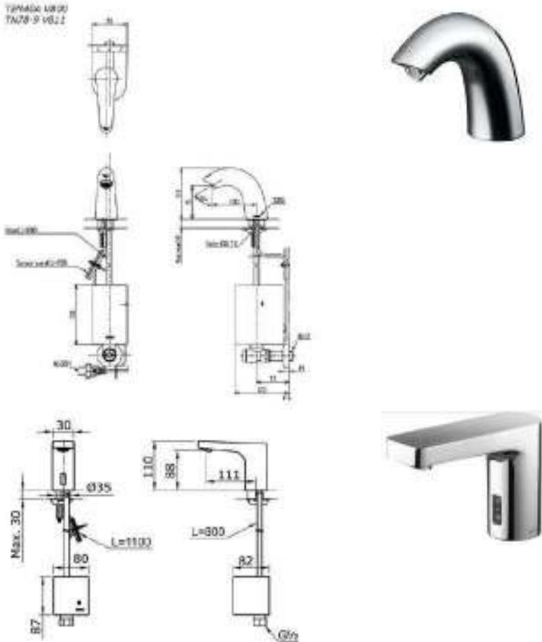
Gambar 4.16 Keran otomatis sensor
